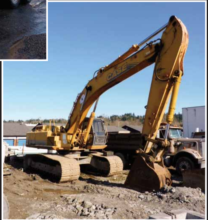
1997 CASE MODEL 9060B HYDRAULIC EXCAVATOR PLUMBED WITH 13' STICK, 36" PADS
