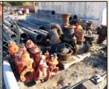
GATE VALVES TEES AND BENDS
