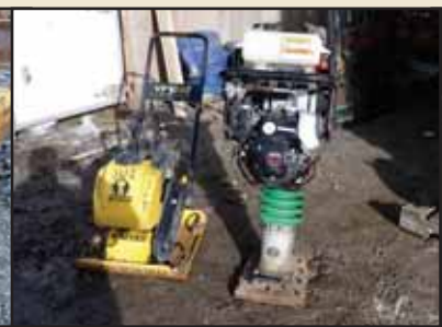
WACKER VP 1550 LOW VIBRATORY PLATE COMPACTOR AND SAKAI RS6 RAMMER COMPACTOR
