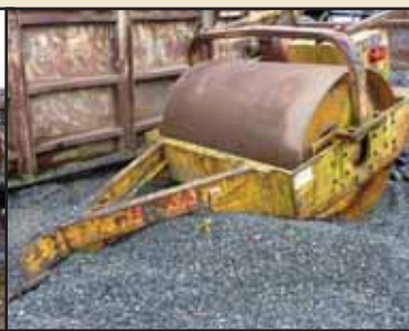
SAKAI MODEL PV20 54" VIBRATORY PULL TYPE ROLLER WITH 1 CYL. GAS ENGINE
