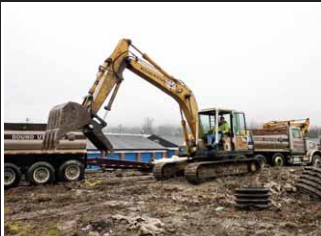
1992 KOMATSU PC120-5 HYDRAULIC EXCAVATOR WITH 8'2" STICK, 24" PADS WITH NEW RAILS AND SPROCKETS
