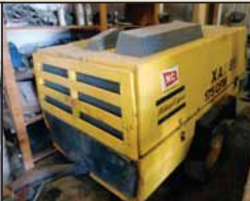
SINGLE AXLE TRAILER CHASSIS, DEUTZ DIESEL ENGINE, COMPRESSOR
