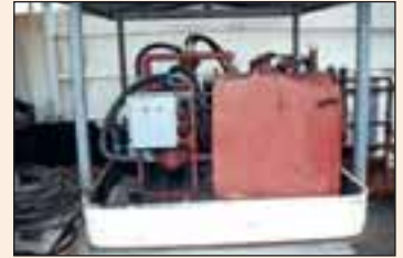
Hydraulic Oil Pump Flushing System With Heater and Pumps
