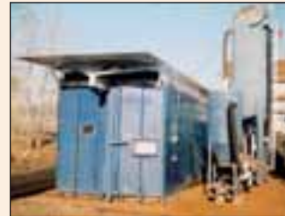
8' x 40' Container Converted to Sandblast Room
